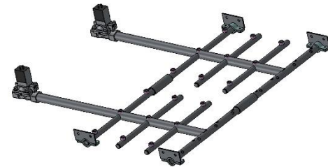
Dutch spiral spray bar for maximizing the surface cleaning.
